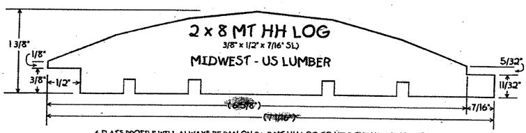
6 Flats profile will always be ran on 2  $\times$  8 MT HH log to Help the Hewning process this pattern is ran down to 13/8. Thick before the Hewning process
